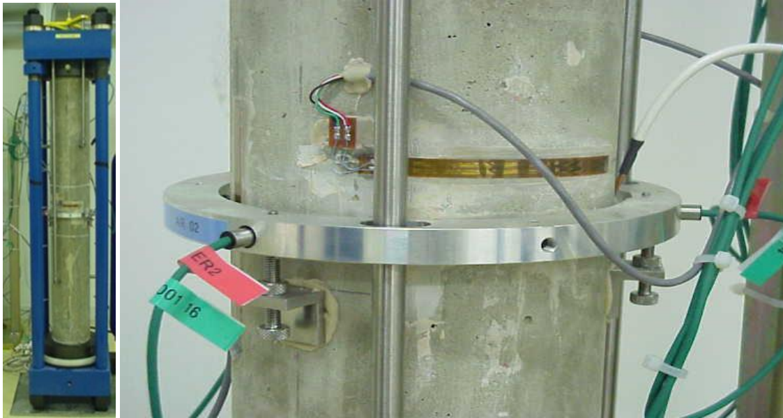
Figure 1. Test arrangement (detail of the center part on the right) [7].
