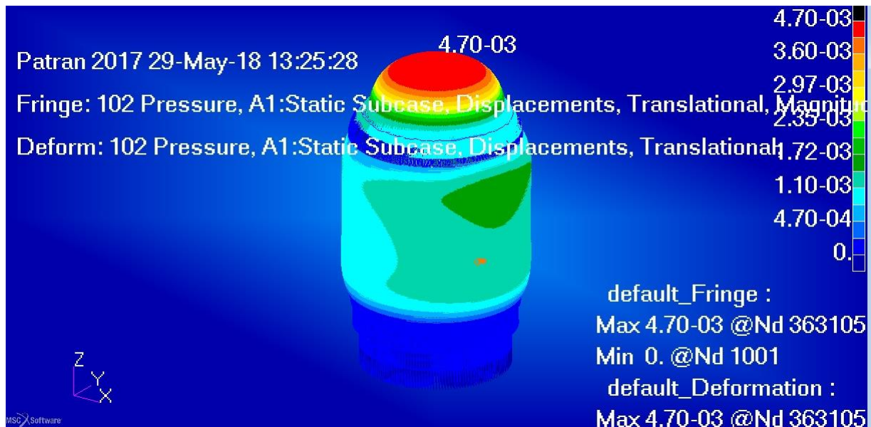
Figure 1. The displacements of of the VERCORS mock-up for the test pressure load case, units are meters.
