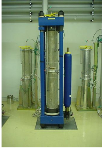
Figure 2: Concrete creep measurement apparatus.
