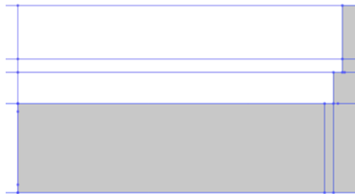
Figure 4. 2D surface representing the gusset and raft in the XY plane.
