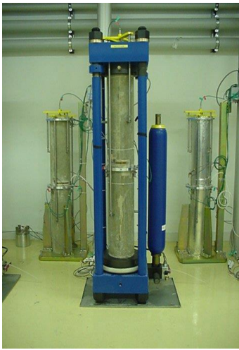
Fig. 3. Concrete creep measurement (VeRCoRs Theme 1)
