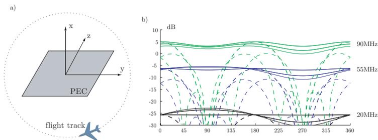
**Figure 7:** Bi-static scattering by a  $(1 + 1)\text{ m} \times 1\text{ m}$  PEC plate for the frequencies 20, 55, 90 MHz. The different curves correspond to illuminating wave field from  $0^\circ$ ,  $45^\circ$ ,  $90^\circ$ ,  $135^\circ$ , and  $180^\circ$ . The vertical (TE) and horizontal (TM) cases are given by the solid and dashed curves, respectively.
