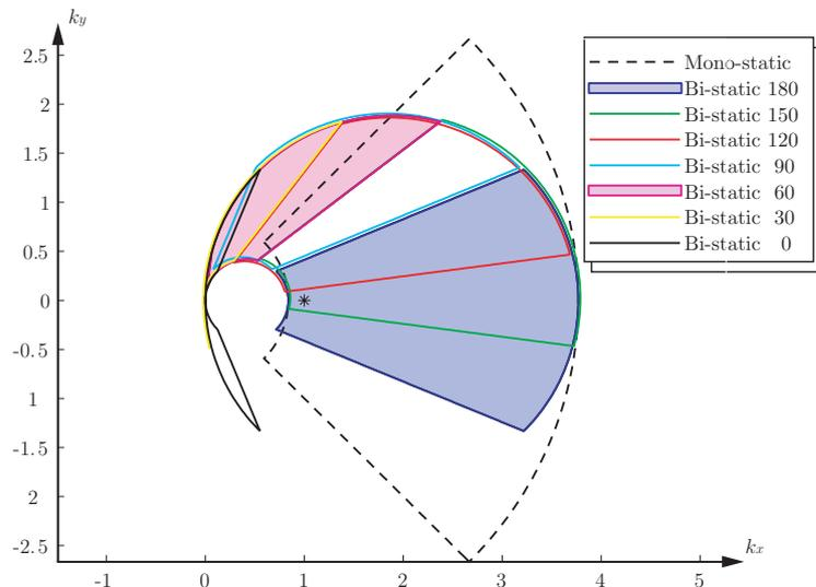
**Figure 2:** Spectral coverage for mono-static and bi-static setups with a  $90^\circ$  aperture angle. The mono-static case has the largest spectral coverage and the spectral coverage of the bi-static cases increases as the scattering angle increases.
