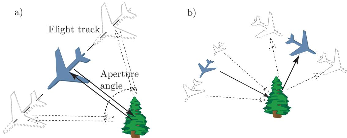
**Figure 1:** Illustration of the SAR setup. a) in the mono-static (backscattering) case, a single airplane is used both to transmit and receive the radar signal. b) in the bi-static case separate airplanes are used as transmitters and receivers. An arbitrary number of airplanes can be used in multi-static cases.
