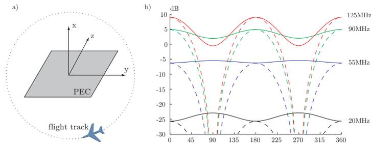
**Figure 5:** Mono-static scattering by a  $1\text{ m} \times 1\text{ m}$  PEC plate for the frequencies 20, 55, 90, 125 MHz. The vertical (TE) and horizontal (TM) cases are given by the solid and dashed curves, respectively.
