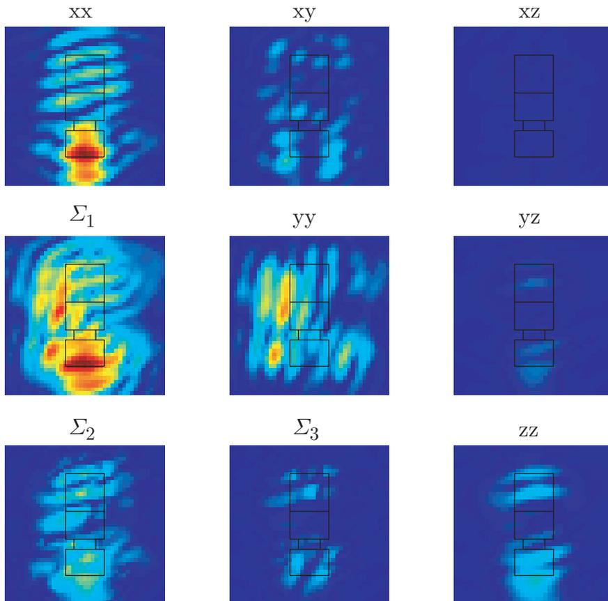
**Figure 8:** Dyadic SAR images from a combined vertically and horizontally polarized case and a flight track given by  $\theta_o = 60^\circ$  and  $100^\circ \leq \phi \leq 350^\circ$ . The horizontal polarization giving the  $xy$ -subspace dominates the image. The  $xx$ - and  $yy$ -components comes from the  $y$ - and  $x$ -directions, respectively. The corresponding SVD images are depicted in the lower triangular part of the matrix.
