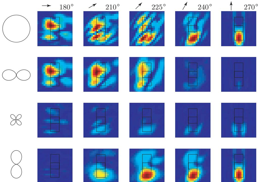
**Figure 3:** Comparison between the SAR images with a point source (top row) and SAR images with a directional dependence. The directional dependence is given by the weight patterns shown to the left of the images. The flight track is between  $180^\circ$  to  $270^\circ$  with an average illumination indicated by the arrows.
