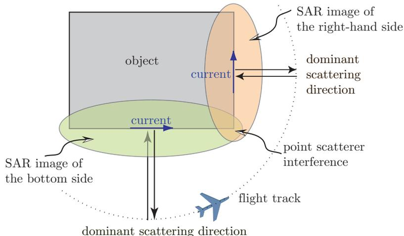
**Figure 4:** Illustration of the point scatter interference. The interference is due to addition of complex valued image parts originating from different scattering processes.
