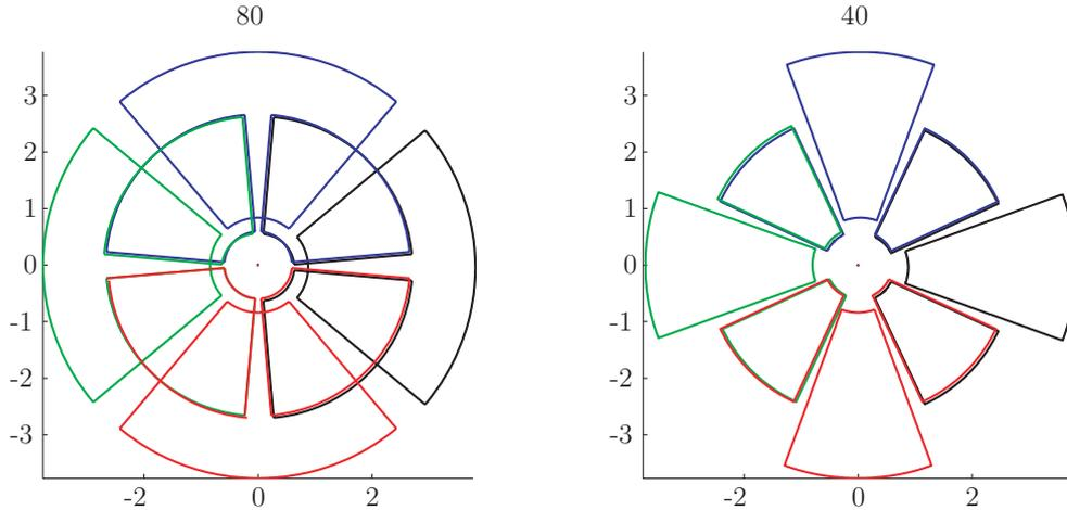
**Figure 16:** The spectral coverage with four transmitting and receiving paths given by  $-\Delta\phi/2 \leq \phi - n\pi/2 \leq \Delta\phi/2$  for  $n = 0, 1, 2, 3$  and  $\Delta\phi = 80^\circ, 40^\circ$ .
