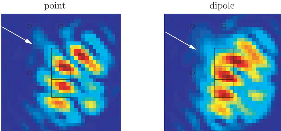
**Figure 12:** Comparison between bi-static SAR images for the point scatter model and dipole scatter model. The vehicle is illuminated with a fixed horizontal wave from an elevation of  $75^\circ$  and azimuth indicated by the arrow. The field is received on a circular path at elevation  $65^\circ$ .
