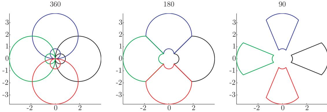
**Figure 15:** The spectral coverage for a multi-static setup with four separate illuminating waves from the azimuth angles  $0^\circ$ ,  $90^\circ$ ,  $180^\circ$ , and  $270^\circ$  and a circular receiving flight path.
