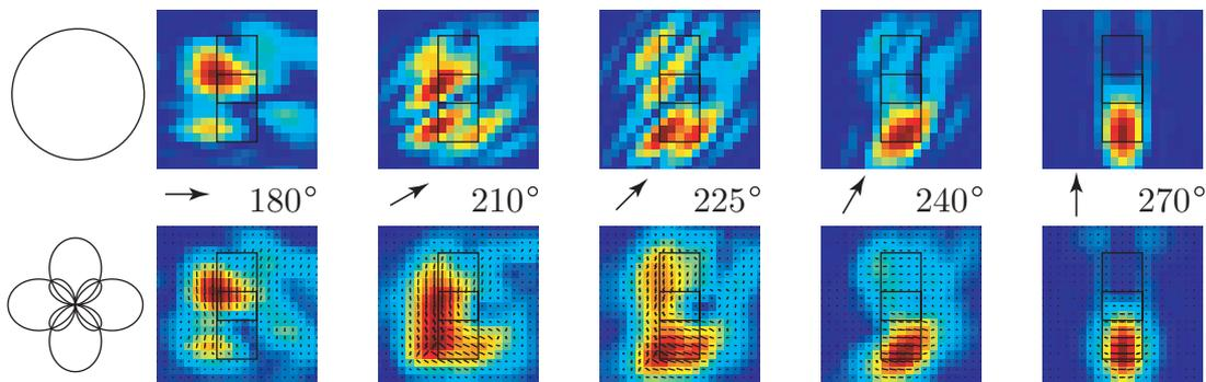
**Figure 10:** Comparison between the SAR images with a point source (top row) and SAR images with an anisotropic source (bottom row). The flight track is between  $180^\circ$  to  $270^\circ$  with an average illumination indicated by the arrows.
