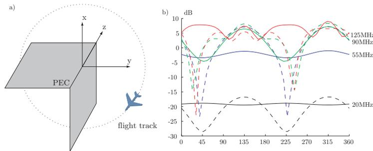
**Figure 6:** Mono-static scattering by a  $(1 + 1)\text{ m} \times 1\text{ m}$  PEC wedge for the frequencies 20, 55, 90, 125 MHz. The vertical (TE) and horizontal (TM) cases are given by the solid and dashed curves, respectively.
