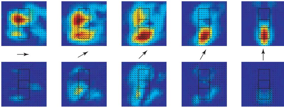
**Figure 9:** SAR images with a with an anisotropic source. The first and second singular values are shown in the first and second row, respectively. The flight track is between  $180^\circ$  to  $270^\circ$  with an average illumination indicated by the arrows.
