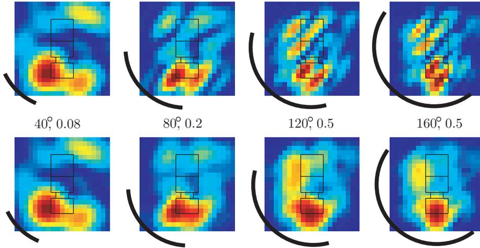
**Figure 11:** Comparison between mono-static SAR images from the point scatter model (top row) and dipole scatter model (bottom row) for the aperture angles  $40^\circ$ ,  $80^\circ$ ,  $120^\circ$ ,  $160^\circ$  as indicated by the circular arcs. The vehicle is illuminated with a horizontal wave from an elevation of  $60^\circ$ .
