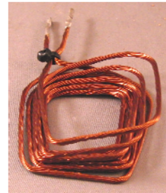
Figure 8: A coil that has lost its shape.
