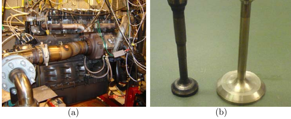
Figure 34 (a) The modified Scania D12 Diesel engine. The operating cylinder is to the left in the picture; (b) Picture illustrating the difference between the “small tank valve” ( \phi = 16 mm) and the “large tank valve” ( \phi = 28 mm).
