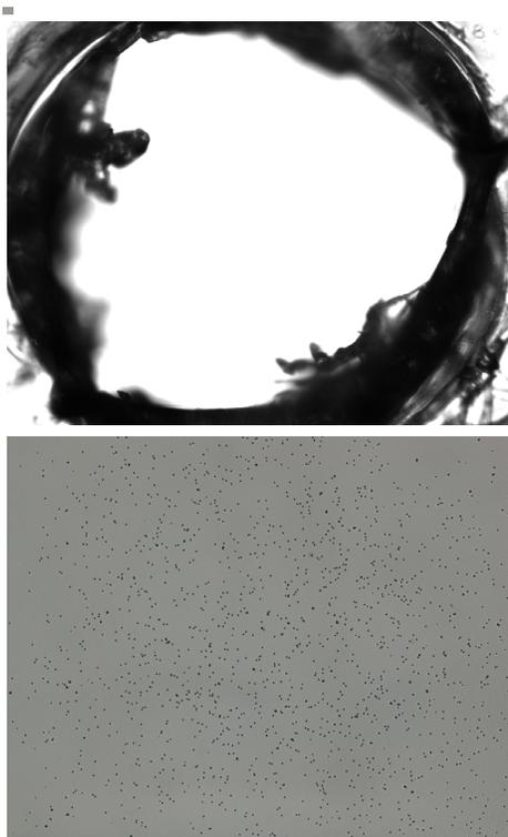
Figure 6.11: Photo ( $10\times$  magnification) of the hole in the Mylar collimator (above) and of alpha particle tracks in CR-39 (below). The diameter of the hole in the Mylar is  $600\ \mu\text{m}$ . The CR-39 was etched for 5 minutes in KOH (12 mol/l) at  $80^\circ\text{C}$  [34]. In the CR-39, only few tracks are visible outside the region shown in the photo.
