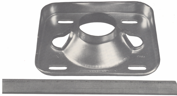
Figure 2.30: Front bumper absorber center mounting bracket formed from 5083-H14 at 250°C [20].
