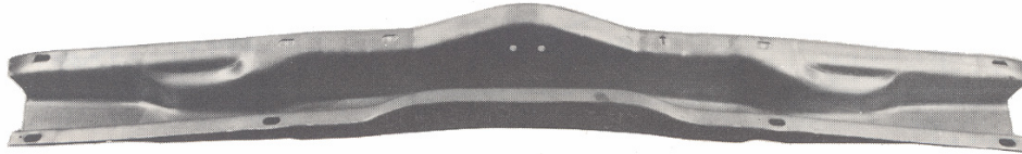
Figure 2.29: Bumper reinforcement formed from 7046-T6 at elevated temperature [20].
