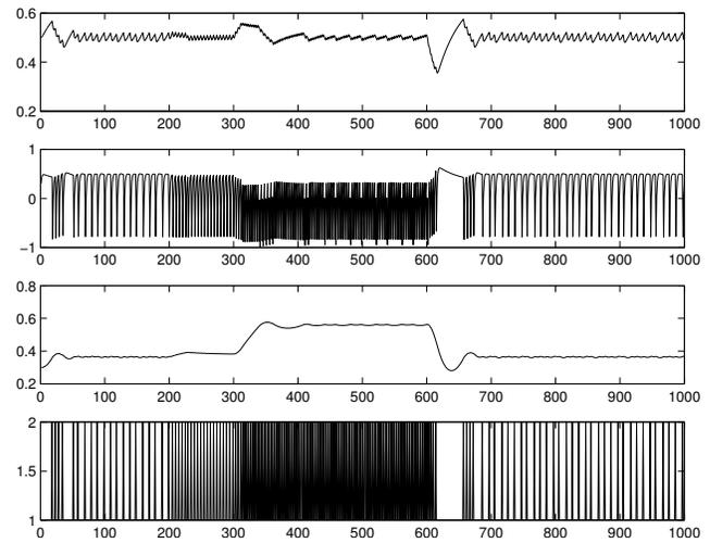
Fig. 3. Top: output voltage. Next to top: current. Next to bottom: integral state. Bottom: Switch position. Reference voltage was  $V_{ref} = .5$ . At  $k = 200$  the load current changes from its nominal value 0.3A to 0.1A, at  $k = 300$  it changes to -0.2A and at  $k = 600$  it changes back to its nominal value 0.3A
