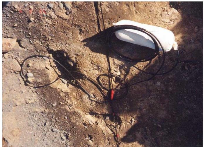
Figure 5. Installation of SP electrodes.
