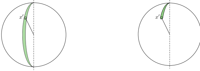
Figure 4.1: The constraints imposed on \bar{x} being the reprojection of the 3D point in first camera. Equation (4.16) constrains \bar{x} to the spherical wedge (left) and (4.15) to the upper part of that wedge (right).
