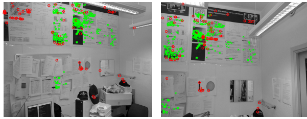
Figure 5.1: Inliers (green) and outliers (red) in a homography estimation. The solution is optimal.
