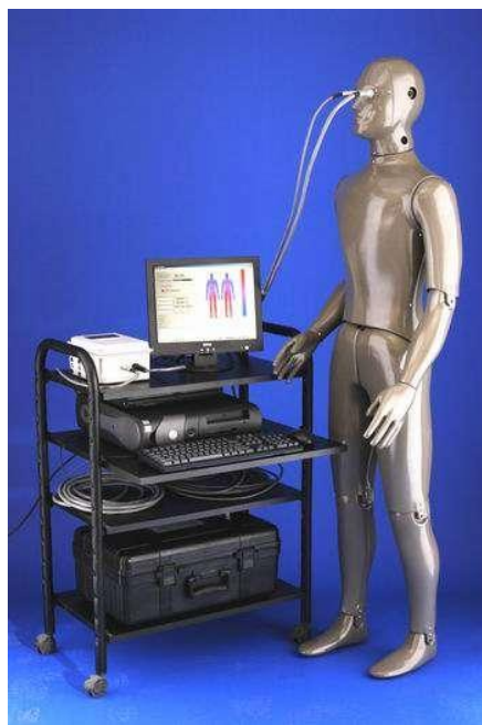
Fig.1 20-zone sweating thermal manikin “Newton”
