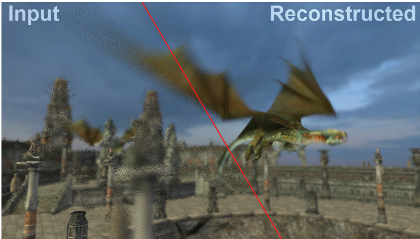
Figure 21: The quality of noisy stochastic renderings can be greatly improved using reconstruction [92].
