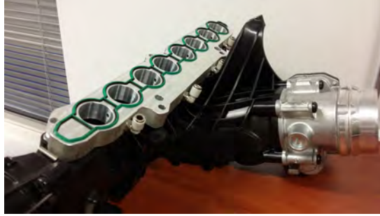
Figure 3.4: Volvo D4 adapter plate for port fuel injection system
