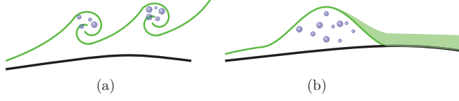
Figure 2.1: (a) The nuclei are trapped in the core of the vortices, downstream the laminar separation. (b) The nuclei are trapped in the small recirculation region, between the laminar separation and the reattachment of the turbulent boundary layer to the wall.
