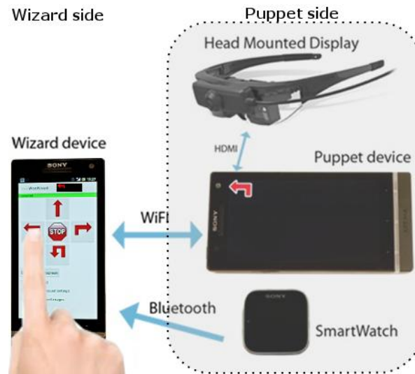
Figure 1: Shows an example of WozARd setup. In this example the wizard use a Sony Xperia S phone while the test person use Vuzix Star 1200, Sony Smartwatch and Sony Xperia S phone. The devices are not in correct scale.
