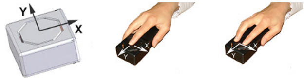
Figure 1. The Viflex device with its octagonal platform (left). The device with its battery extension handle can be used with one (middle) or two (right) fingers.
