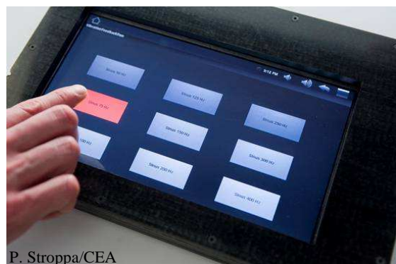
Figure 2. Modified ARNOVA 10 G2 tablet with a housing including the compliant frame and the piezoelectric actuator.
