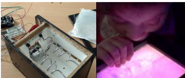
Figure 1. Left: Open LivelyButton showing metal spirals, LED-strips and motor components. Right: child interacting with the LivelyButton.
