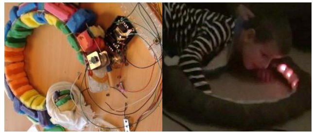
Figure 2. Left: Internal structure of the LivelyForm. Right: Child interacting with the LivelyForm, showing a capacitive sensing outer side with a semi-transparent lit inner side.
