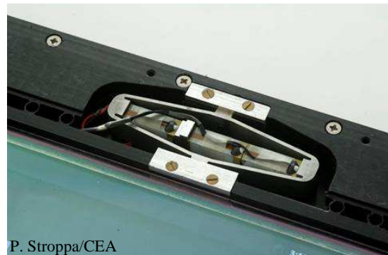
Figure 1. Touch screen integrated into a compliant structure powered by an amplified piezoelectric actuator.
