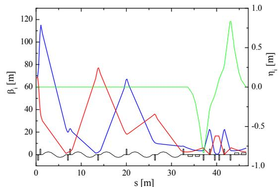
Figure 1: Horizontal (red) and vertical (blue) beta functions and vertical dispersion (green) along the linac and transfer line starting from 2<sup>nd</sup> accelerating structure.
