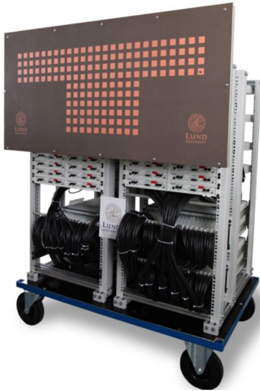
Figure 3.10: The Lund University Massive MIMO testbed.
