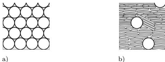
Figure 4.1: Idealisation of a granular and clayey soil where white represent solid particles and grey fluids. a) granular soil. b) clayey soil.
