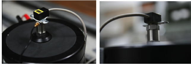
Fig. 4. Details of the fixation of the MEMS to the reference accelerometer and the shaker.
