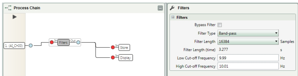
Fig. 5.3: Filter used in B&K PUSLE REFLEX environment.
