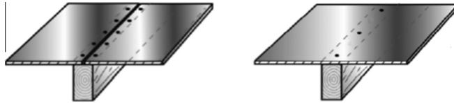
Fig. 1. Dual-plate junction (left) and single-plate junction (right).
