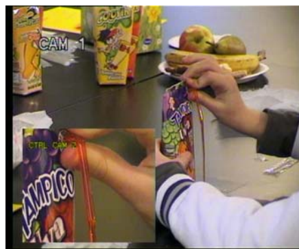
Figure 5.2 Leakage from the straw
