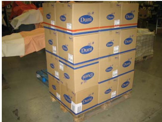
Picture 4.3.3b A unit load with an adhesive tape strip in Bramsche. 176
