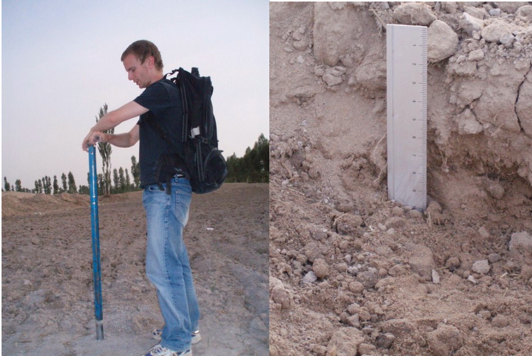
Figure 18. Extracting soil samples by drill. The ruler was used to get to the correct depth.
