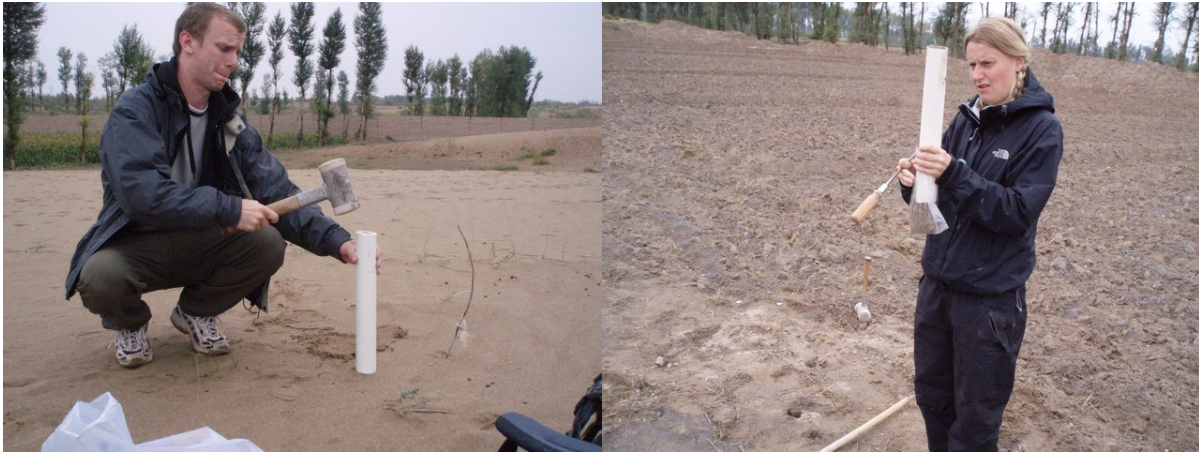
Figure 16. Collecting soil samples with a PVC tube.
