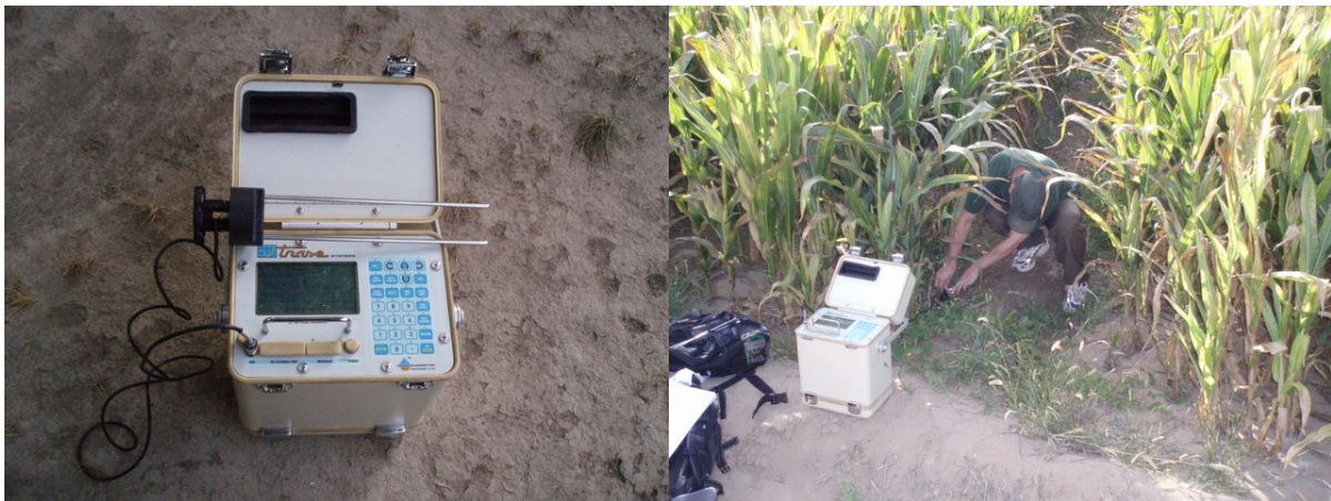
Figure 15. The Time Domain Reflectometer with its waveguides and TDR usage in cornfield.
