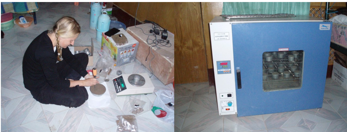
Figure 17. The scale and oven used for water content determination.
