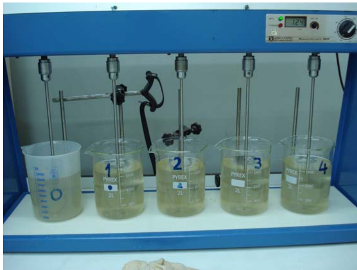
Figure 6. Jar test equipment in action.
