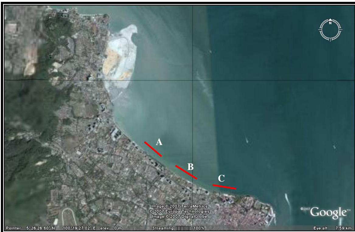
Figure 23 : Shoreline stretches at locations A, B and C used to study local sediment transport pattern before and after the land reclamation
