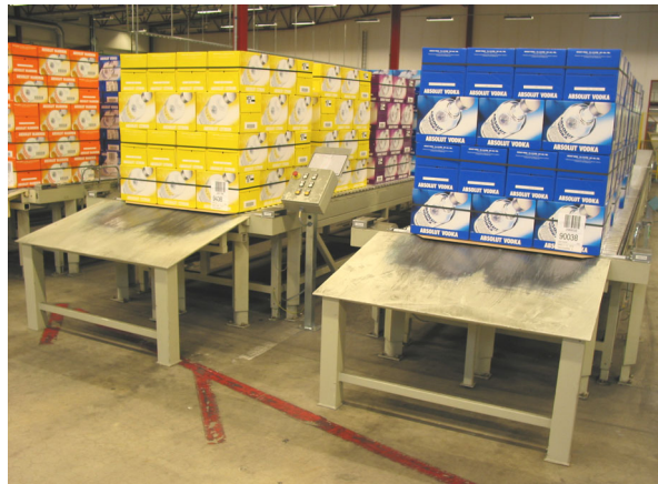
Figure 54: Slip Sheet packages placed in front of a trackpad in order to facilitate handling.
