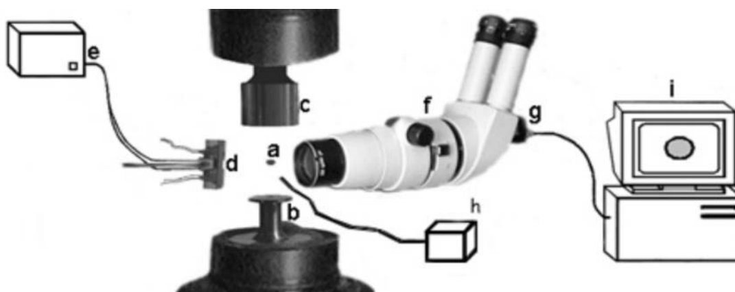
Figure 8: Overview of the instrumental setup: a) a levitated droplet, b) the transducer of the levitator, c) the reflector, d) the flow-through dispenser, e) power supply box for the dispenser, where slope and amplitude are chosen, f) represents the objective, g) the camera, h) the RALS system, i) the computer.
