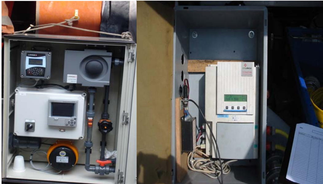
Figure 11 - Two different models of Dr. Lange turbidity meters (Kjellberg, 2006). This equipment can easily be attached inside the vehicle.
