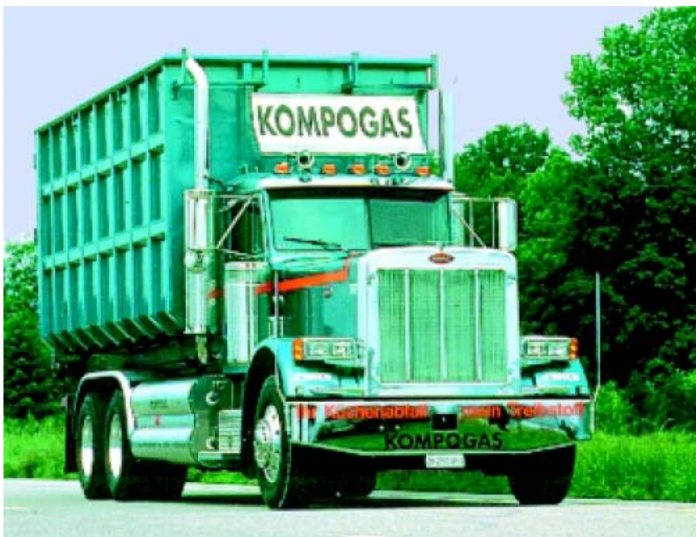
Figure 2-9 Biogas powered truck for collection of waste at the Kompogas facility
