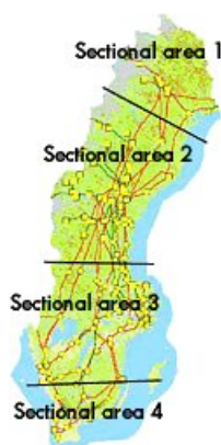
Figure 2-3 Division of the Swedish electricity supply network into sectional areas
