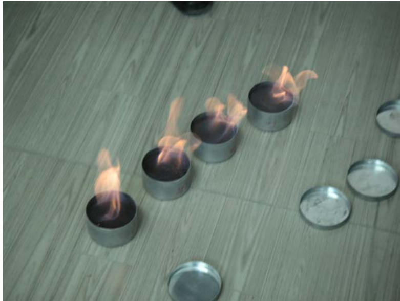
Figure 3.2 Drying up the soil-samples with conventional method (Cheung, 2006).
