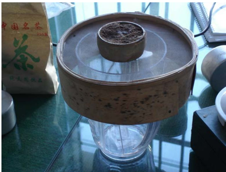
Figure 3.5 A soil sample on top of a filter measuring field capacity (Schjånberg, 2006).
