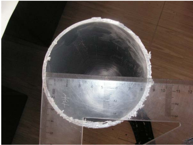
Figure 3.3 Pipe for infiltration test (Cheung, 2006).
