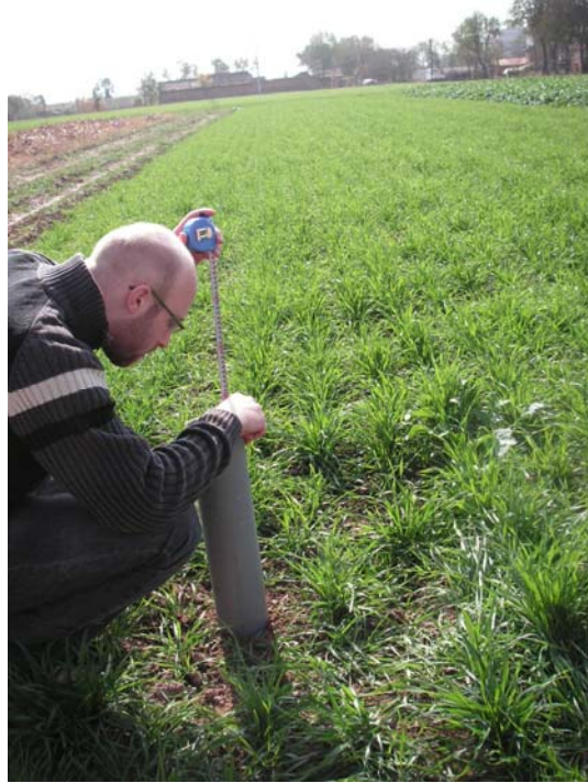
Figure 3.4 Measuring water level in the infiltration pipe (Cheung, 2006).
