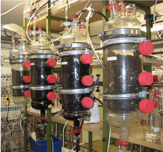
Figure 25 Four bioreactors used for landfill simulation. From right to left: Reactor 1, aerobic, reactor 2, anaerobic with leachate recirculation, reactor 3, anaerobic and reactor four, anaerobic dry
