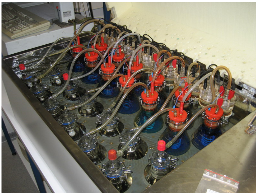
Figure 3 Photo of reaction vessels, oxygen generators and manometers of a Sapromat at the Institute of Waste Resource Management at TUHH
