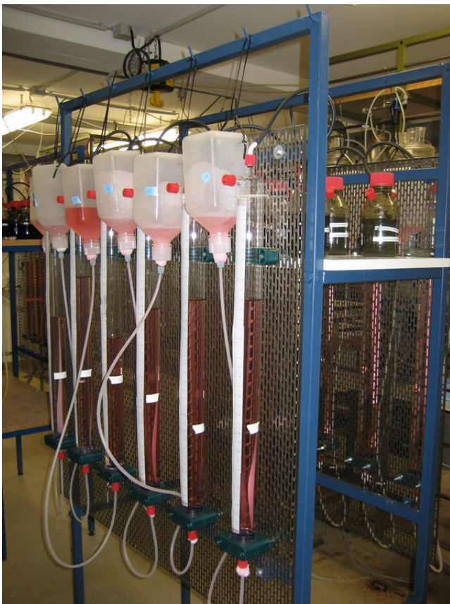
Figure 5 Photo of the anaerobic test system used to assess the gas formation potential
