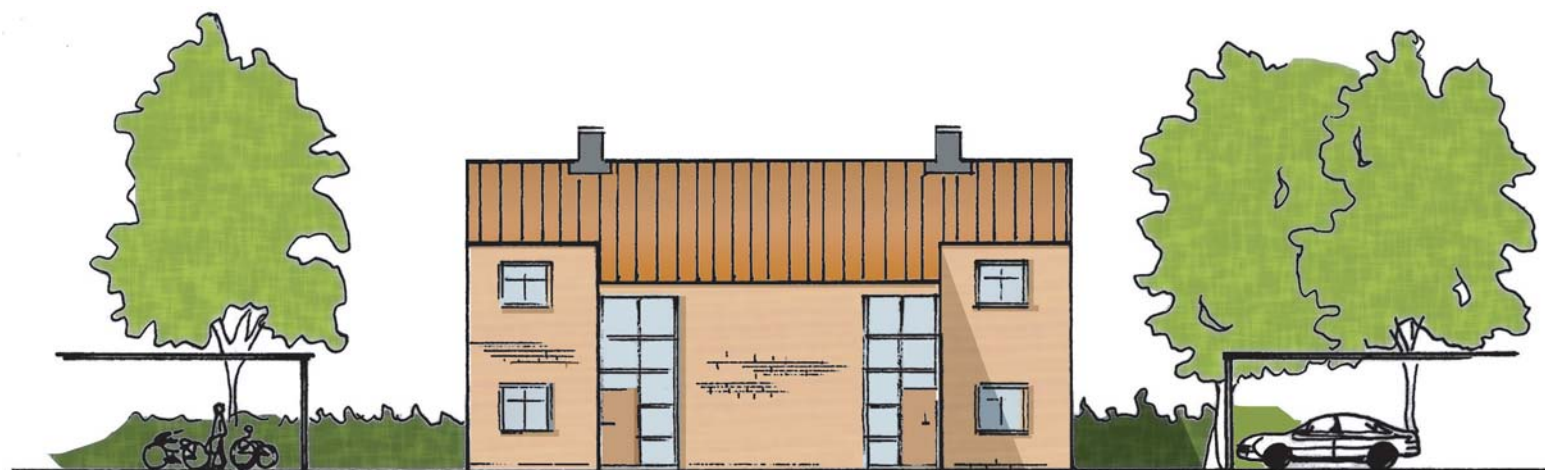
Semidetached houses - reused bricks 1:200
