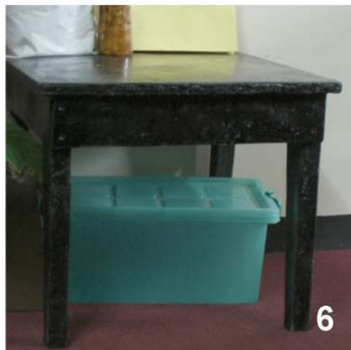
1-6 Recycling of soft plastics at Los Baños Eco-Waste Processing Centre. The collected plastics (1) are melted by person wearing protection equipment (2), then put into a mould (3) and pressed (4) in order to create hard plastic sheets (5) that can for example be used for tables (6). (Karolina Huss 2006-05-19)
