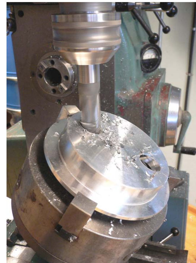
Fig. 62. Milling operation for foot piece.
