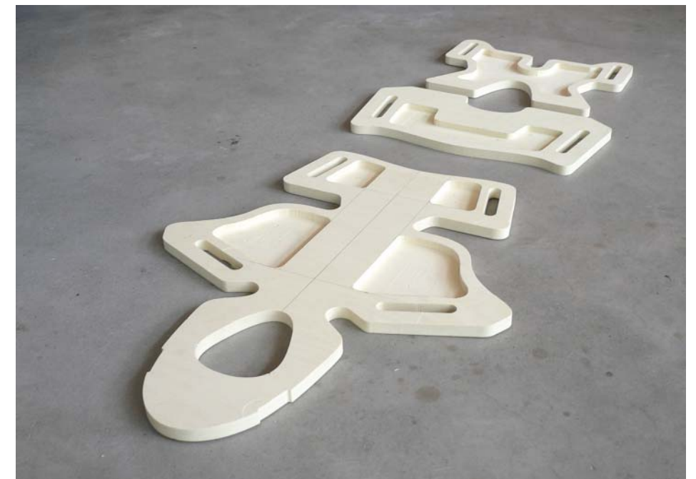
Fig. 58. Boards after milling the compartment for the foam.
