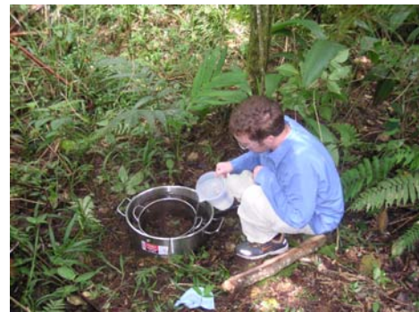
Figure 7. Double ring infiltrometer setup
