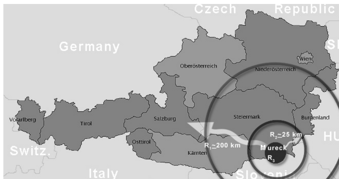
Figure 3-4 Collection systems and average catchment radii. R_1=200\text{km} corresponds to the collection of UFO, R_2=25\text{km} corresponds to the collection of rapeseed and R_3=5-8\text{km} corresponds to the collection of resources for Ökostrom (adapted from Bio-energy Cycle Mureck, 2005).
