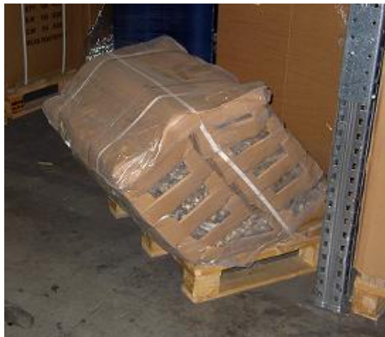
Figure 5.2. Unstable pallet that has become askew.
