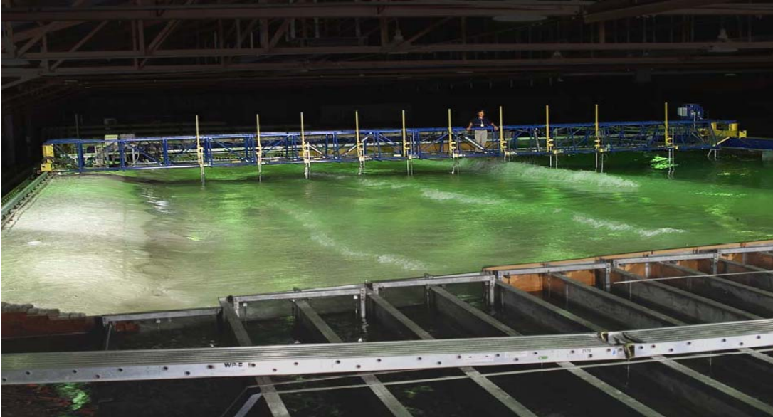
Figure 2.2 An experiment on longshore sediment transport conducted in the LSTF. 7
