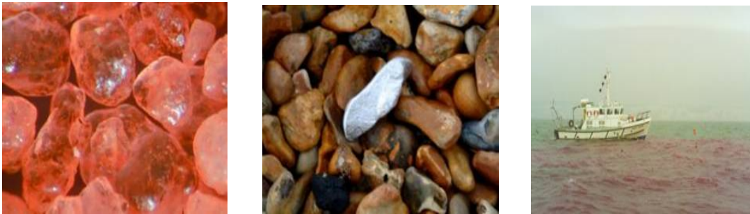
Figure 2.1 From the left, an example of sand tracer, viewed under a low magnification microscope, a shingle tracer in use in a littoral environment, and a dye-and-drogue tracking study. 6
