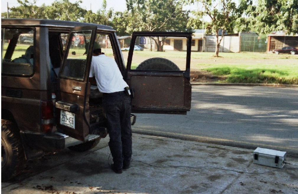
Figure 5.9 The sensors are lowered from the rear compartment of the jeep at the arrival at the site. In this picture only the accelerograph has been placed on the sidewalk.
