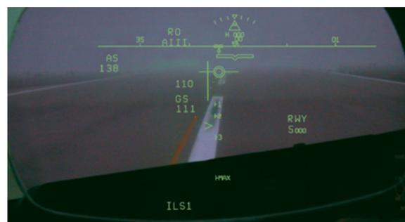
Tailstrike protection is generated through a pitch limit symbol that first appears on the top of the pitch scale and then translates downwards. Tailstrike protection can be used with or without the FD activated during take off. Upon landing the pitch limit symbol is replaced with a large letter “TAILSTRIKE” warning across the center of the display. The need for tailstrike protection is becoming more and more important as aircraft body length extends [6].
