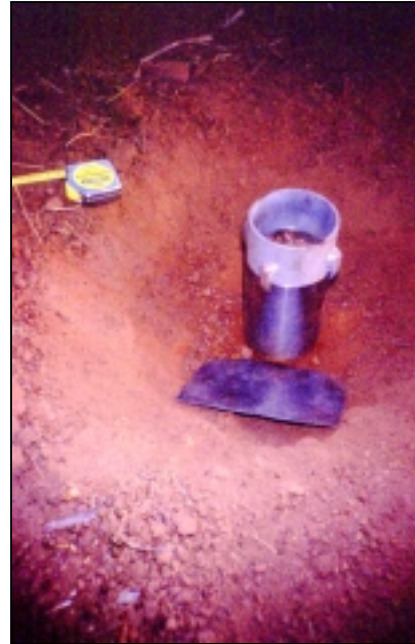
Figure 4.8. At the bulk density sampling a steel plate was inserted beneath the cylinder.
