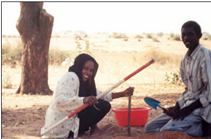
Figure 5.3: The interpreter and the driver during soil sampling: with the stick (in the sample hole) we measured the depth and with the spade I scratched along the side of the hole to receive the soil. Then we mixed the sample in the bowl and put around 50 g into a plastic bag.
