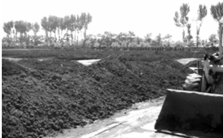
Figure 11 Long rows with sludge that are being composted at Daxing Sludge Disposal Plant. The loader to the right is used to turn the piles over.
