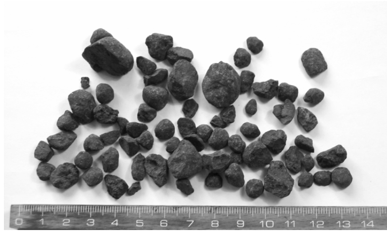
Figure 13 Processed sludge that are ready to be used as constructing material. Hard pebbles in the size between 4-12 mm.
