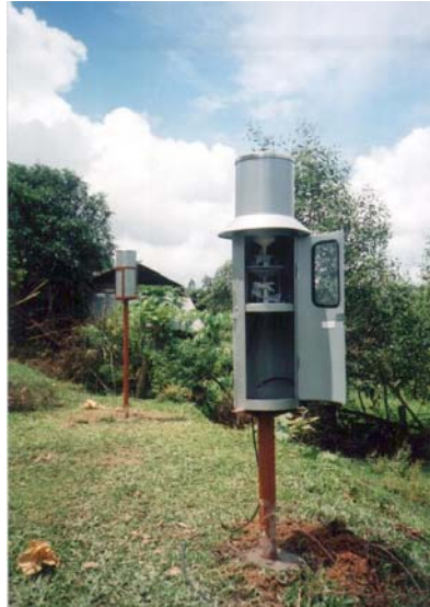
Figure 2.2.1: Rain gauges used for the measurements in Lo Dong catchment area (Ali-Maher et al, 2004).
