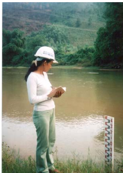
Figure 2.2.3: Water level measurement in Lo Dong (Ali-Maher et al,2004)
