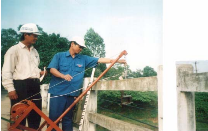
Figure 2.2.2: Water current meter in Hoa Phu (Ali-Maher et al, 2004)
