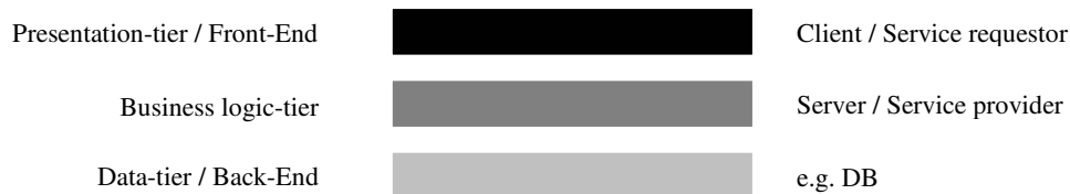
Figure 21: A three-tier client/server or service requestor/service provider architecture, disregarding that requestors might also occur on the Business logic-tier. (Inspired by: Hammerschall, 2005)
