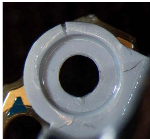
Figure 6.11 – Cracks in the loop in the PCB
