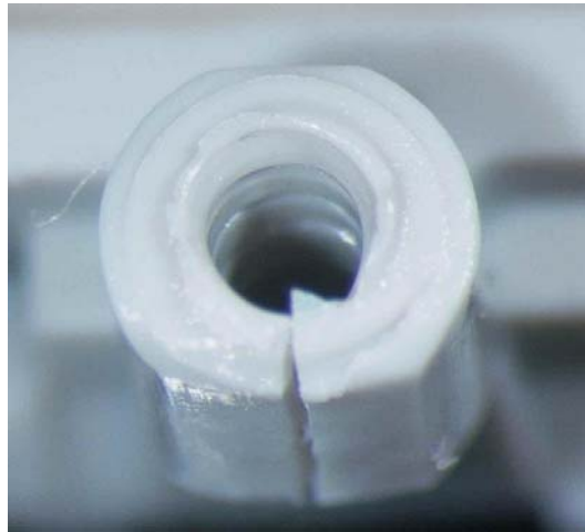
Figure 6.9 – Crack in the 1.4 mm screw boss
