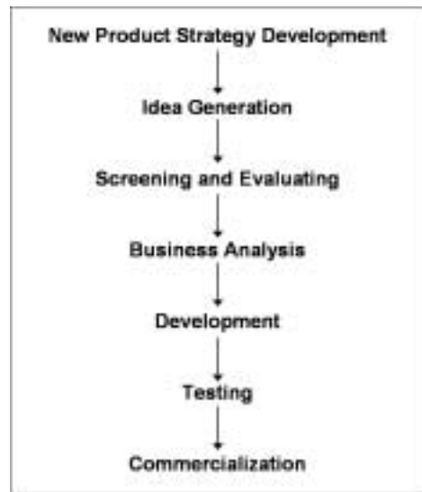
Figure 6.1 – New product development according to the consulting firm of Booz, Allen and Hamilton from 1982. The model is an improvement of their earlier model containing an additional phase; New Product Strategy Development. (Scheuing & Johnson, 1989)
