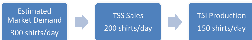
Figure 11: A system approach disclosing the TSI production as the total system's bottleneck.
