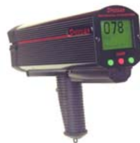
Figure 2.3 Radar gun used for speed measurements
