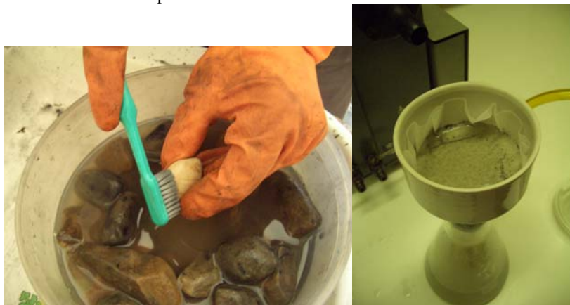
Figure 32. Left: Washing stones to do biofilm evaluation. Right: Filtering wash water using a vacuum pump.
