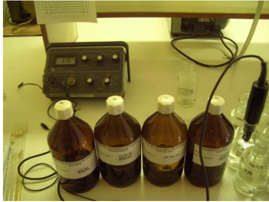
Figure 30. Bottles with nutrients for the microorganisms in the BOD 5 test and equipment for measuring oxygen content.
