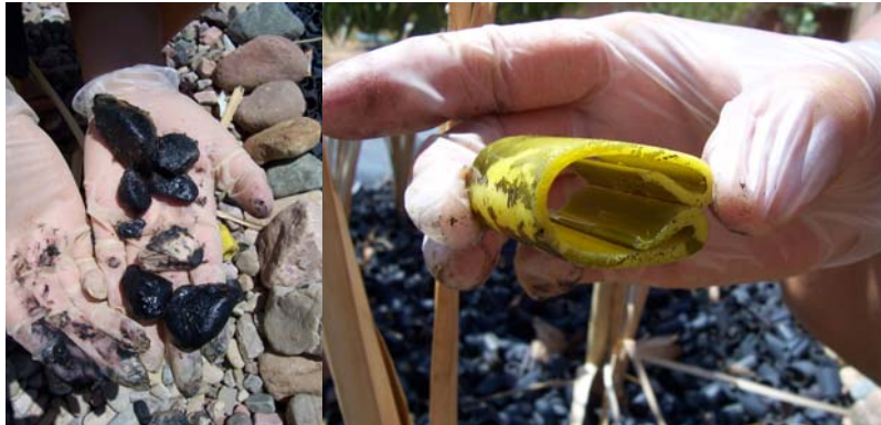
Figure 44. Biofilm and residue from the wastewater can be seen on stones (left) and plastic (right), excavated from just below the water surface.
