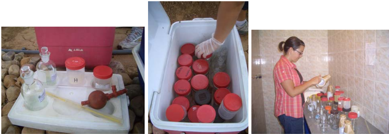
Figure 28. Left: Analyses equipment ready to be used in the field. Middle: Filled containers were placed in an insulated, dark box. Right: Helena is inspecting and marking the containers at the laboratory.
