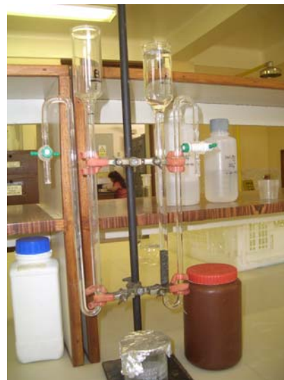
Figure 29. Equipment for reducing nitrate with cupperized cadmium granules.
