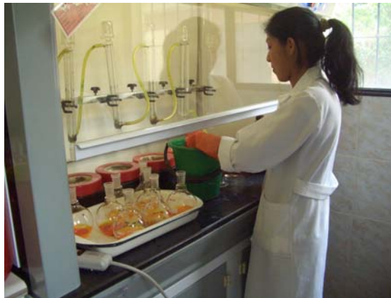
Figure 31. Staff at C.A.S.A. adding sulfuric acid as a part of the COD analysis.
