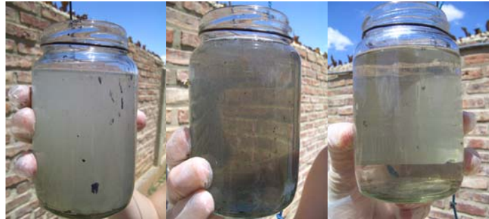
Figure 43. Left: septic tank. Middle: 4 th stone chamber. Right: 7 th plastic chamber.
