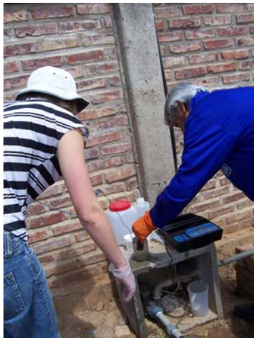
Figure 27. Sofia and our supervisor Marcelo Ledezma, measuring conductivity.
