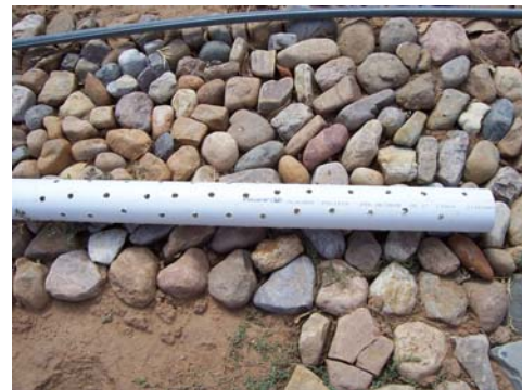
Figure 25. New observation pipe with drilled holes, ready to be installed in the wetland.
