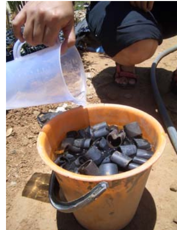
Figure 24. Porosity measurement of the plastic medium.
